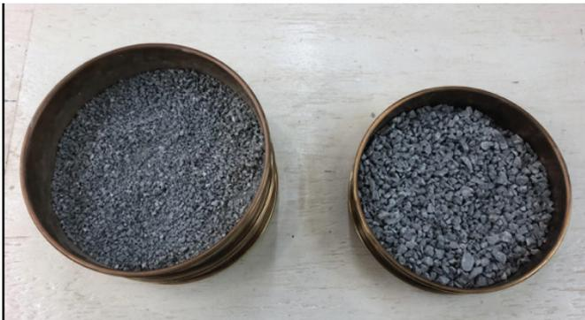
Figure 6. Soapstone sorted into two size classes using geological sieves
